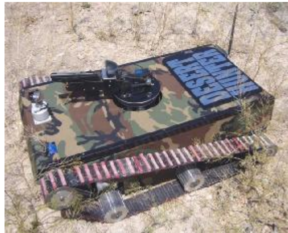
Figure 1: Desert Hunter: Military tracked robot for surveillance and reconnaissance applications
